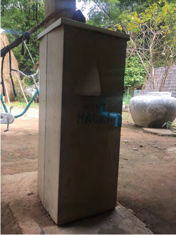
The smaller scale “at home” version of the BioSand filter.
